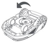
5. Remove the blade by aligning the hole of the blade with the shaft.
