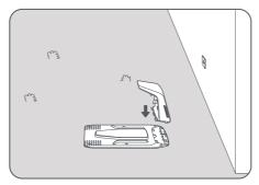
3 Insert the cleaning brush into the charging tower by aligning the tongue with the groove.
