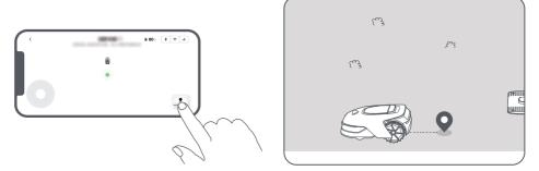
**3** Remote control A1 to move along the edge of your lawn to create the work area. When remotely controlling A1 to create the boundary, please bear in mind:
