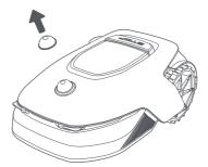
Press Stop button to open the cover of the control panel. Press and hold the Power button on the control panel for 2 seconds to turn on A1.
