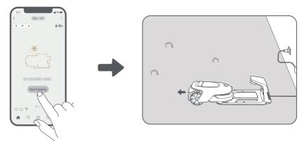
Remote control A1 to the edge of your lawn and tap "Set Starting Point" to confirm the starting point of the boundary.
