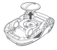
2 Remove the LiDAR protective cover.
