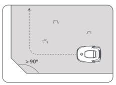
When A1 returns to the place 1 m near the starting point, you can tap "Close Boundary" and the boundary will automatically be completed.
