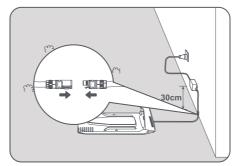
**6** Put A1 in the charging station to charge. Make sure the charging contacts on A1 and the charging station are connected correctly.
