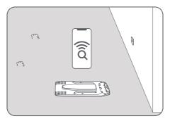
• Keep at least **1m** of free space with no obstacles to the left, right and in front of the charging station. Make sure that the grass around the location is shorter than **6 cm**. If the grass is taller, please mow it with a push mower first. Tall grass may make it difficult for A1 to return to the charging station.
