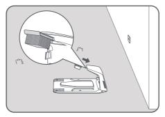
Onnect the power supply to the extension cable and then connect to a power outlet. Please keep the power supply at least 30 cm above the ground.
