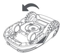
4. Clean the body of A1, blade disc and chassis with a hose.
